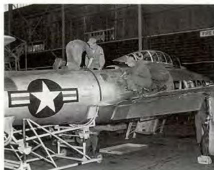
"Bloody-knuckle" technology was the order of the day as these F-84G mechanics could readily attest. Sharp edges on panels caused a big share of grief for the unwary or inexperienced.
